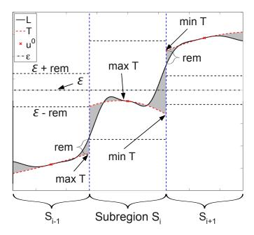
Figure 1. One-dimensional illustration of the reliability verification of a constraint L with a Taylor polynomial of second order in a subregion  $S_i$ .
