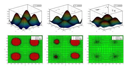
Figure 2. Iteration of the learning algorithm. Green boxes show regions where the constraint is verified, red boxes where the constraint is violated and crosses mark samples in U obtained by the iteration process. The maximal output bound is strongly violated by the unconstrained learner (left). The output of the network shrinks in each step of the iteration (center). The constraint is satisfied and proofed (right).
